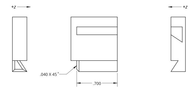
All leading edges of tab to be chamfered. Optionally, chamfer leading edges of slot.
